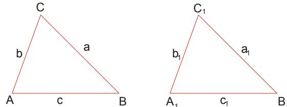
$$\triangle ABC \cong \triangle A_1B_1C_1 \Leftrightarrow a = a_1 \wedge b = b_1 \wedge c = c_1$$
